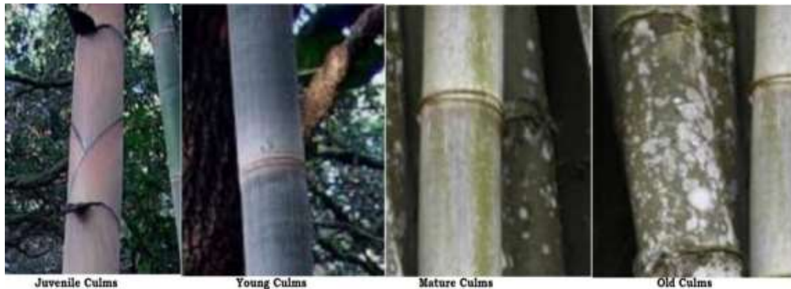
Figure 2.1: Bamboo gradually changes from the outside
